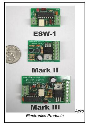
Replacing it are two new products. The first is the all new Mark II Ignition Unit. This is a standalone unit and does not include the ESW-1. The major feature is the protection afforded the output transistor and ignition coil in the event the engine stops prematurely with the points closed. If this happens, the unit shuts down immediately protecting the unit from possible overload and the ignition coil from burning up. It measures approx. 1-1/8 x 1-1/2 inches.
